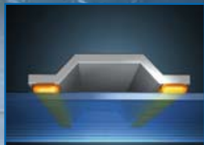
Bonding of back rails
